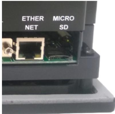
There is an Ethernet port available on the EZ TouchPLC. This port enables users to add/update programming through an Ethernet connection. It allows for both PC and PLC simultaneous communications. It can also be used for Internet access and email alerts.
