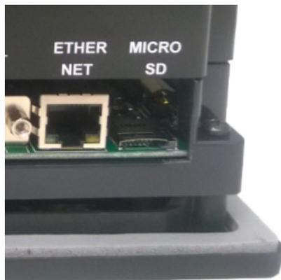
A Micro SD slot is available for data logging purposes. Additional details about using a MicroSD Card for data logging is available in the [Data Logging Overview](#) section. Push against the Micro SD card to eject it from the TouchPLC unit when finished.
